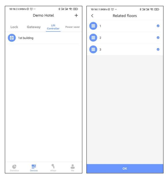
Configure floor information to lift controller, and set the working mode.
