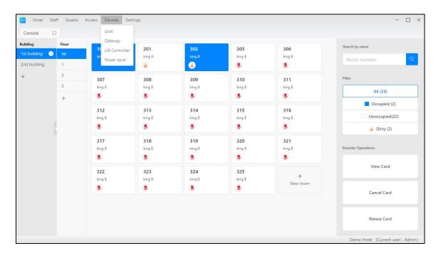
Manage locks, gateways, lift controller and power saver here.
